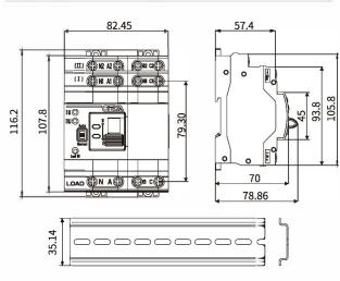
Note: Terminal wiring area: fit for (1~25)mm<sup>2</sup>. Wire connection screw is M5, torque: 2.5N.m.
